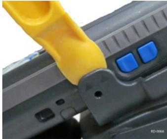
**Figure 6. Separating computer from scan handle**
