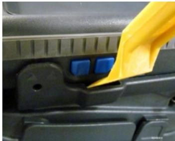
**Figure 7. Slide implement into channel**
