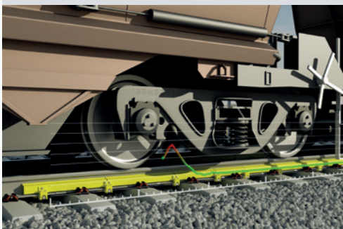
Flat wheel detection system
