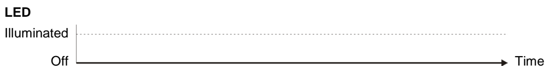
Figure 10.3: LED “Sys1” and/or “Sys2” off
