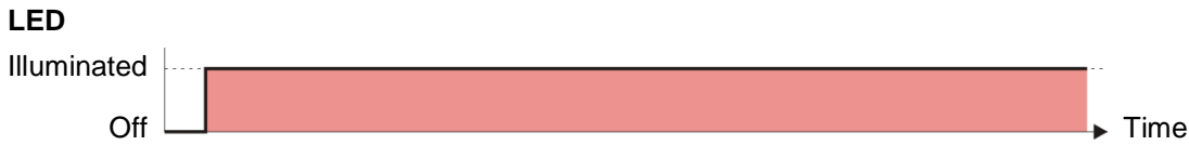
Figure 10.4: LED “Sys1” and/or “Sys2” illuminated
