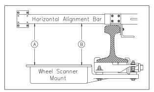
The transducer height bracket on the bottom of the alignment fixture can be used to ensure proper installation of the transducers. When the transducer body touches the bracket, the transducer body is 1-9/16 inches (3.97 centimeters) below the top of the rail <u>and</u> parallel to it.
