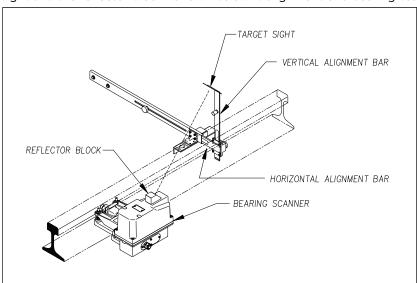
To align wheel scanners, you use the horizontal alignment bar of the fixture. Alignment is done by measuring from the bottom of the extended bar to the top of both ends of the scanner mount. When both measurements are the same, alignment is correct. That is, as shown below, when distance **A** is <u>equal</u> to distance **B**, alignment is correct.
