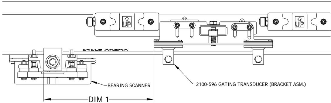
Loosely mount the bracket on the rail then slide horizontally as necessary so that DIM1 is the correct distance for your rail size. DIM1 (see above) is the distance from the far edge of the track clamp on the bearing scanner to the near edge of the bracket assembly. Using the tables below, note the distance for your rail size. Tighten the nuts to 35 ft lbs.
