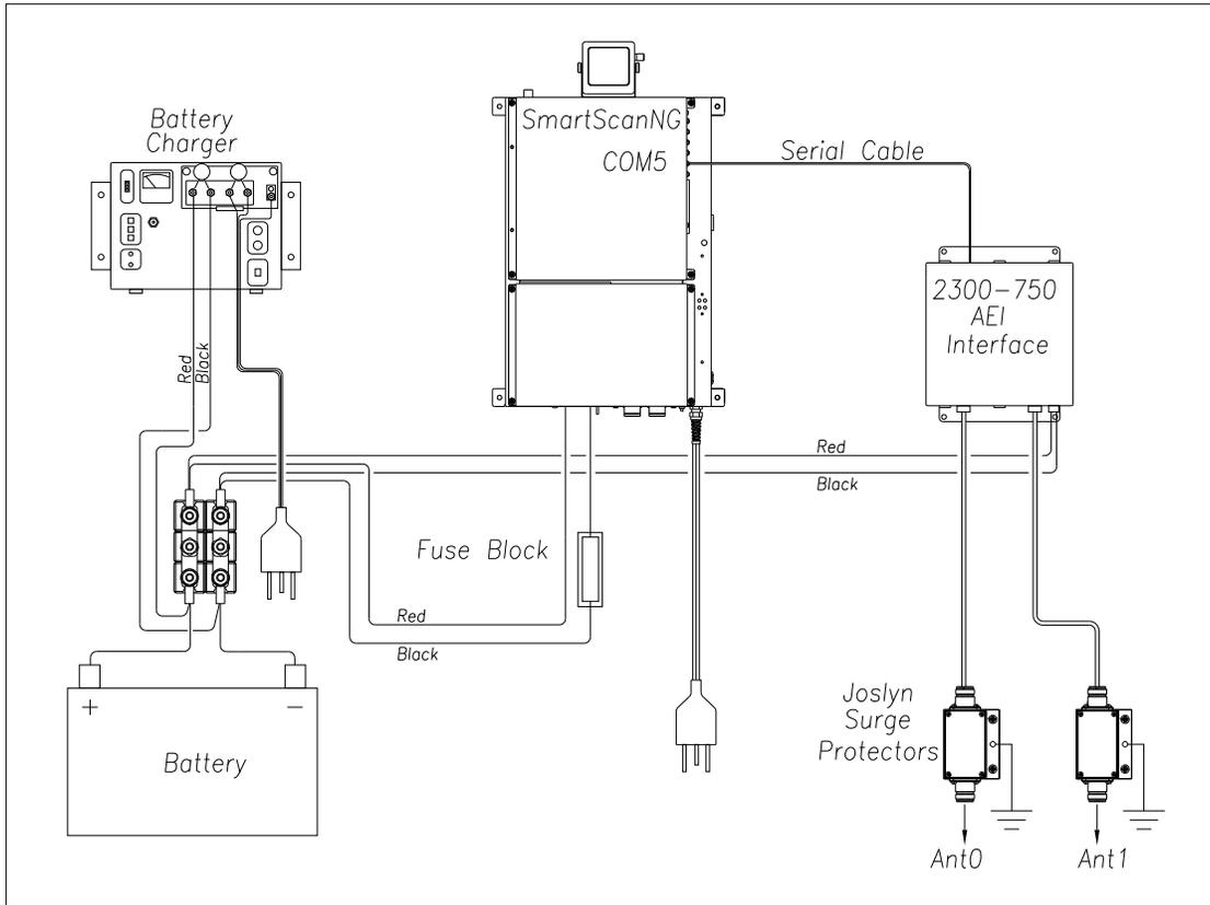
The AEI Interface module (2300-750) chassis should be tied to earth ground. To do this, connect a ground wire to the ground connector on the mounting tab on the AEI Interface module. Any size copper wire can be used for grounding. Instead of wrapping the wire around the ground connector, either crimp a ring terminal to the grounding wire before slipping it onto the ground connector or slip a copper ground lug onto the ground connector and use it to hold the grounding wire.
