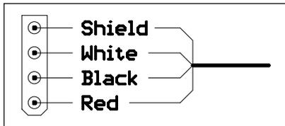
The red wire supplies 12 VDC to the shielded temperature probe.
