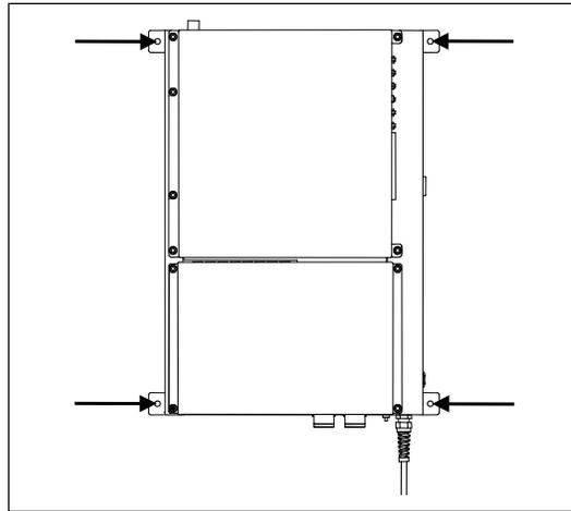
Mount the SmartScanNG enclosure about 4 feet (1.2 meters) above the floor. Doing so positions the enclosure at a convenient height for installation and servicing. Mounting it at this height also allows you to install the power subsystem below it.
