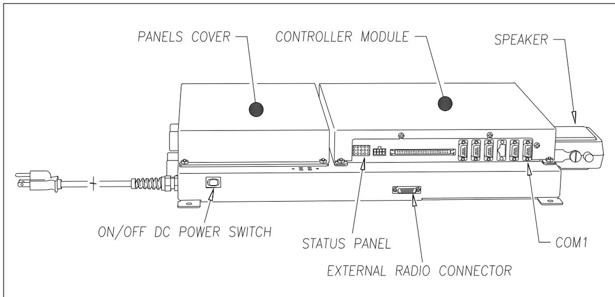
The power cord at the bottom of the SmartScanNG enclosure is used to power the heaters in the 2500-512AC scanner. This cord should be plugged into a grounded three-wire 120-volt outlet. Minimum operating voltage is 110 volts. **Plugging the cord into an outlet of more than 128-volts will severely damage your system.**
