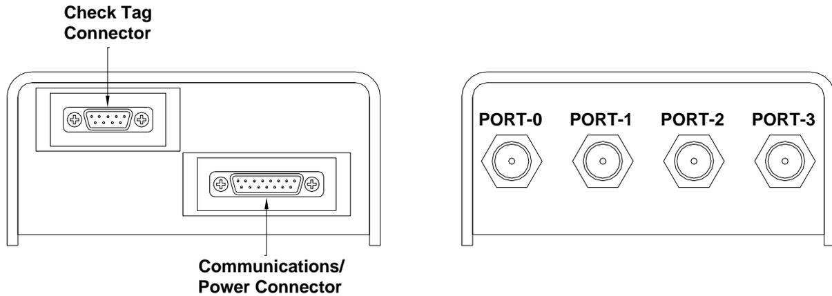
Power and serial communications are brought in through the DB15F connector.
