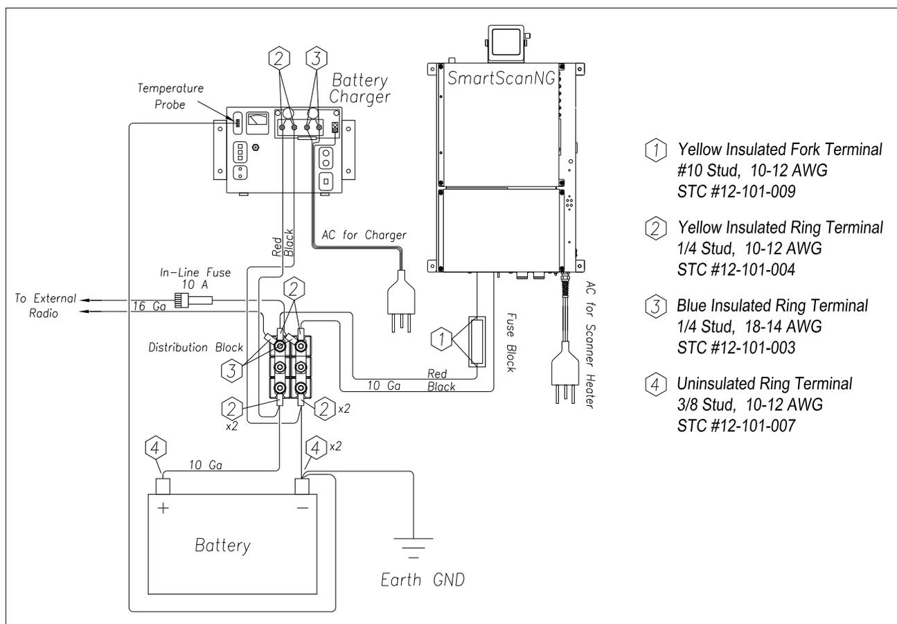
There is one SmartScanNG enclosure per track. One power subsystem per SmartScanNG enclosure. One battery per power subsystem. One battery charger per battery.
