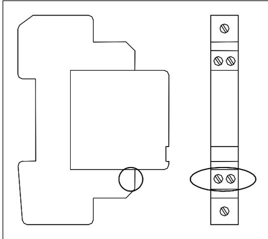
Each UTB is mounted horizontally on a DIN rail. Shown to the left are two views of the same UTB.
