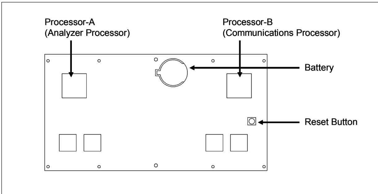
The Processor board uses two, independently operating, central processing units (CPUs). The CPU on the left (aka processor-A aka Analyzer Processor) is responsible for data retrieval from external sources, such as the shielded temperature probe, scanners, transducers, and auxiliary devices. The CPU on the right (aka processor-B aka Communications Processor) is used to process and store the data retrieved by the other CPU. It then presents information to the user in the form of reports.
