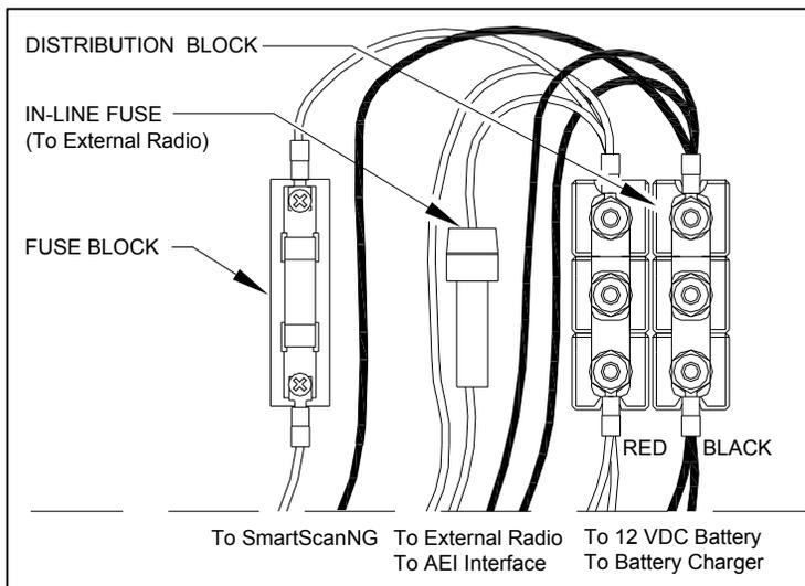
The **distribution block** contains six terminals. Loosening the middle gold nuts will disconnect DC power to the rest of the system. Wires from the bottom of the distribution block go to the 12V battery and to the battery charger. Wires from its top go to the fuse block, to the AEI Interface, and to the external radio.
