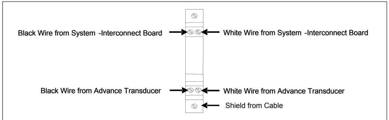
**Observe correct polarity** when you connect the wires from the transducers. The polarity is correct when the transducer's white wire is connected directly below the existing white wire at row two of the UTB, and the transducer's black wire is connected directly below the existing black wire at row two of the UTB. Connect **ADV1** first and **ADV2** second. **ADV1** is the advance transducer to the right of gating transducer **TO2**. **ADV2** is the one to the left of gating transducer **TO1**.
