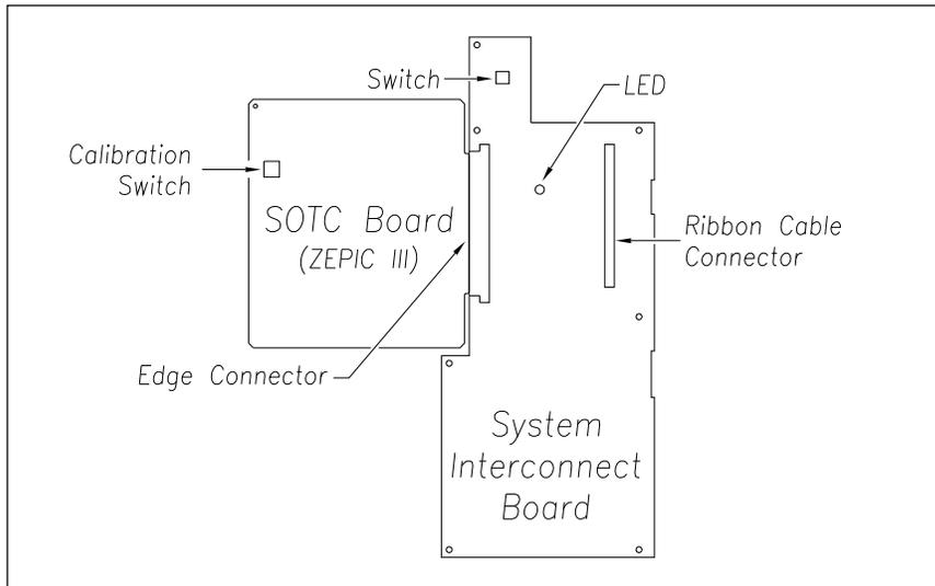
5. The relay drive will pick up (LED on) when the unit has successfully calibrated. This process can take up to 45 seconds to complete.
