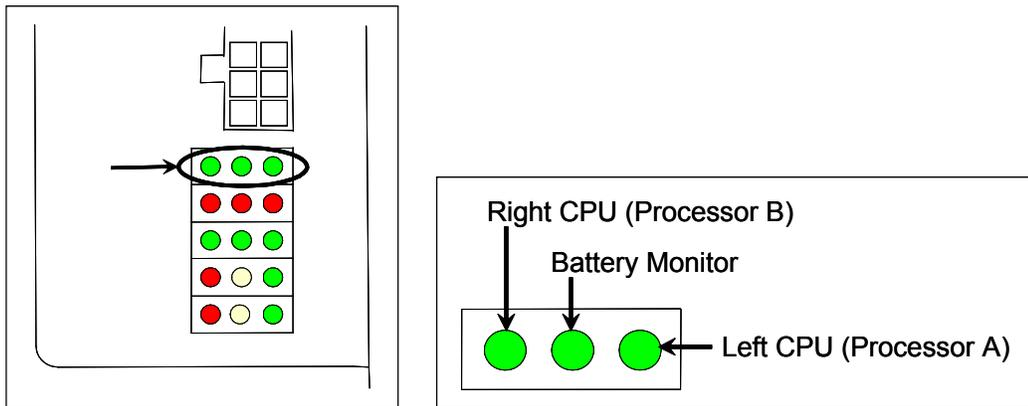
The top row of green LEDs indicates the condition of the CPUs and the battery on the Processor board. If both CPUs are running their programs correctly, their LEDs pulsate (that is, repeat the cycle off, dim, bright, dim). If a program isn't operating as expected, the LED for the affected CPU blinks on and off, is lit solid, or isn't lit at all.
