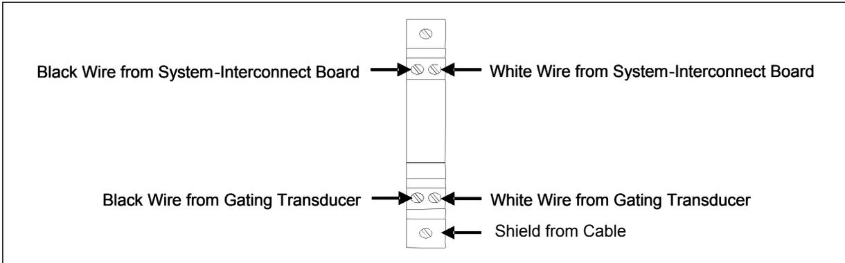
**Observe correct polarity** when you connect the wires from the transducers. The polarity is correct when the transducer's white wire is connected directly under the existing white wire at row two of the UTB, and the transducer's black wire is connected directly under the existing black wire at row two of the UTB. Connect **TO1** first and **TO2** second. **TO2** is the northmost or eastmost gating transducer.
