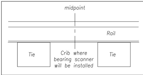
If you are going to install antenna masts, in addition to identifying where the bearing scanners will be installed, this midpoint mark will also be used later to locate where the holes for the mast bases are to be dug.
