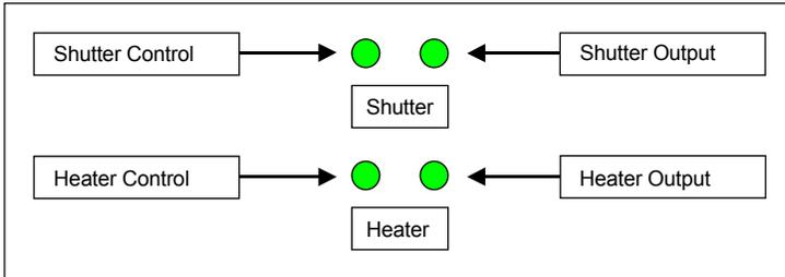
Not all four LEDs can be lit at the same time. Anytime the shutters are open, the heaters should be off. Under normal conditions, the top two LEDs (shutters) should only be lit when the heaters are off. Conversely, under normal conditions, the bottom two LEDs (heaters) should only be lit when the shutters are closed. In other words, when the system is working, only the top two LEDs are lit when a train is rolling through the site. When no train is present, only the bottom two LEDs may be lit.
