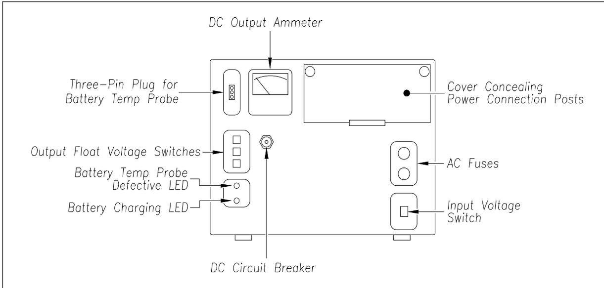
The input voltage switch can be set to 115 VAC or 230 VAC. Use 115 for input voltages between 108 and 128. Use 230 for input voltages between 216 and 256.
