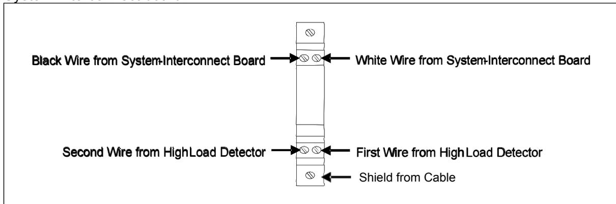
Correct polarity need not be observed when connecting the wires from the high-load/high-wide detector. One wire from the detector should be connected directly below the existing white wire at row two of the UTB, and the other wire should be connected directly below the existing black wire at row two of the UTB.
