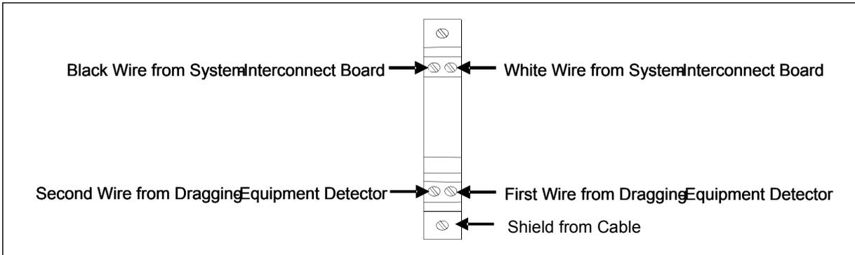
Correct polarity need not be observed when connecting the wires from the detector. One wire from the detector should be connected directly below the existing white wire at row two of the UTB, and the other wire should be connected directly below the existing black wire at row two of the UTB.
