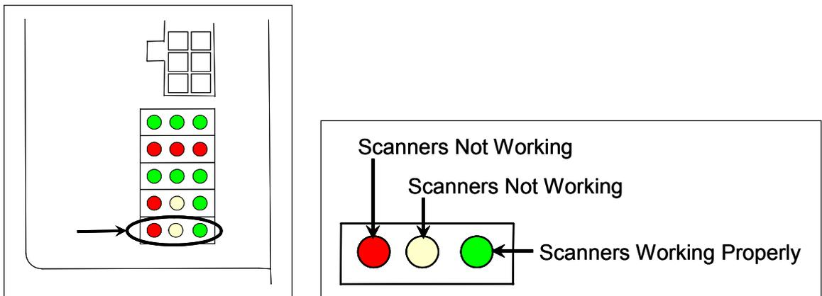
The leftmost red LED indicates whether the integrity check passed or failed. If a scanner failed integrity on any of the last 20 trains, this LED lights and remains lit until all trains with integrity failures are flushed from the log. Conditions that would trigger the lighting of this LED are:
