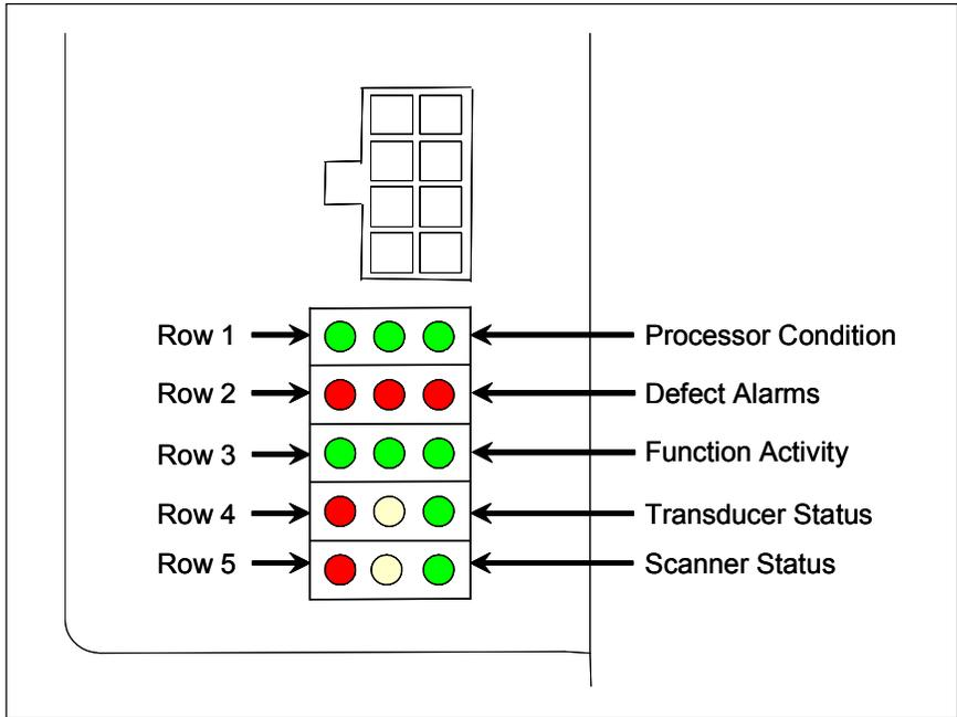
The information that is used to control rows 4 and 5 is contained in a log of the last 20 trains to pass the site. A separate log of the last 40 trains controls the LEDs in row 2. Both of these logs clear at power-up or reset.
