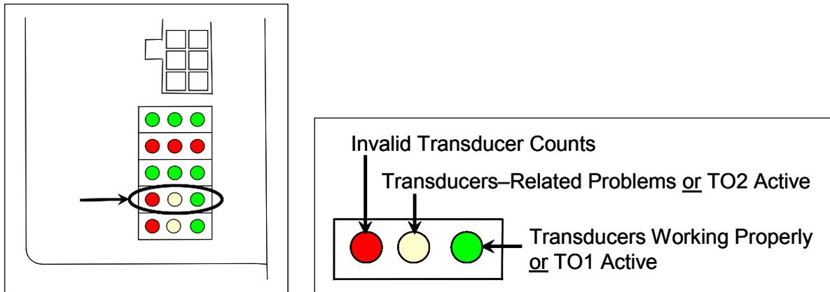
When a train is present at the site, this row indicates the operational status of the gating transducers for the current train. The rightmost green LED will flash as a wheel travels over transducer TO1. The center yellow LED will flash when a wheel travels over transducer TO2. The leftmost red LED doesn't light during train passage, except when both transducers fail integrity tests.
