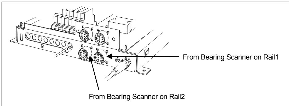
**3** Plug the connector from the bearing scanner on rail2 (that is, from the south or west rail) into the leftmost box connector on the backmost part of the bottom of the SmartScanNG enclosure.
