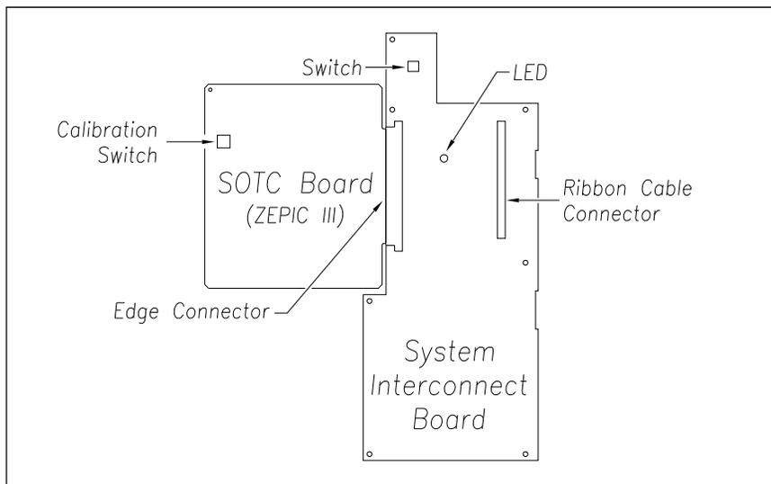
The SmartScanNG enclosure only has a SOTC board if the site is using a track circuit. If the site is using two advance transducers, there is no SOTC board.
