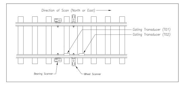
The **<u>type2</u>** wheel scanners are aligned to scan about 4 inches (10.2 centimeters) above the rail.
