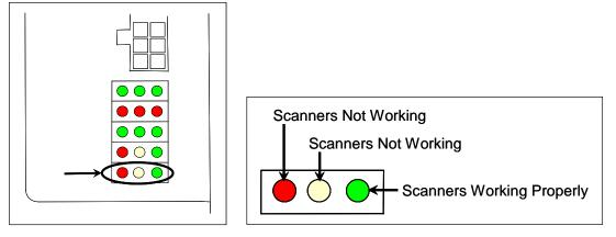
The bottom row of LEDs indicates the operational condition of the bearing and wheel scanners when the system is at rest (that is, when a train isn't present at the site). Several conditions are monitored and logged.
