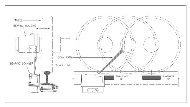
Bearing temperatures are sampled for a short period before the gate opens, to support detection of Pyrometer Saturation alarms, and while the gate is open.
