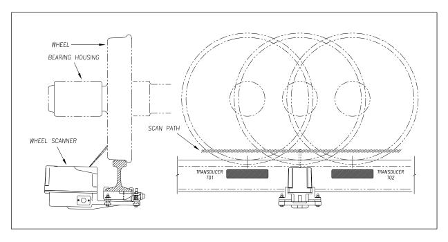
The SmartScanNG system checks for hotwheels during the scanning process.
