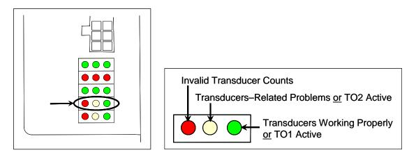
On the Interface board (in the Controller module), the transducer signals undergo RF filtering and amplification with a gain of 30. For validation, the amplified signals are fed into comparators, which create 5-VDC pulses lasting the period of time that the amplified signals remains above 620 millivolts. Processor-A (on the Processor board) receives these 5-VDC pulses through ports PA0 (TO1) and PA1 (TO2).
