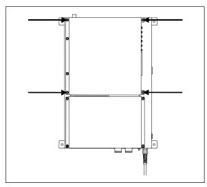
**d** Detach the Controller module from the rest of the SmartScanNG enclosure.
