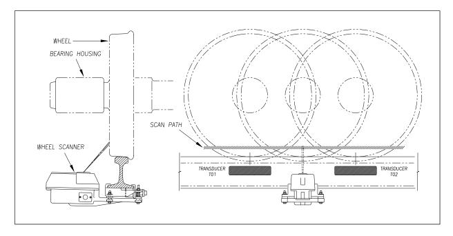
The **type3** wheel scanners are aligned to scan about 4 inches (10.2 centimeters) above the rail.
