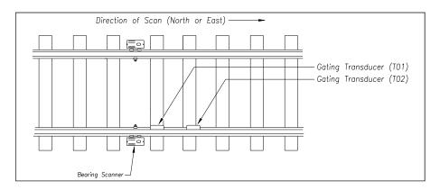
The **type2** bearing scanners are aligned to scan the bottom 3.5 inches (8.9 centimeters) of the bearing housing, about 7.25 inches (18.4 centimeters) from the gauge line.
