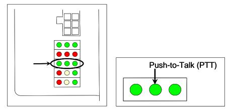
If this LED isn't lit, the system's ability to send a message to the radio might be inhibited by the **Radio Inhibit option** on the System Functions menu. If the radio is inhibited, the results of this check are invalid.
