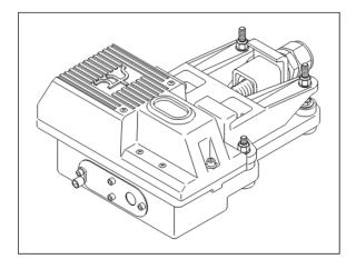
An assembled **<u>type3</u>** bearing scanner looks like this.
