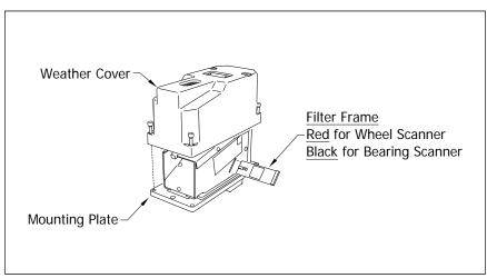
You'll need to remove the weather cover before you can replace the filter frame. Four socket-head-cap screws attach the weather cover to the mounting plate. Before continuing, be sure that the <u>black</u> filter frame is securely in place and that the four socket-head-cap screws on the weather cover are completely tight.
