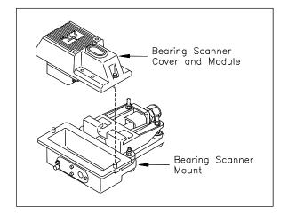
The figure below shows the major parts of a **<u>type3</u>** bearing scanner.
