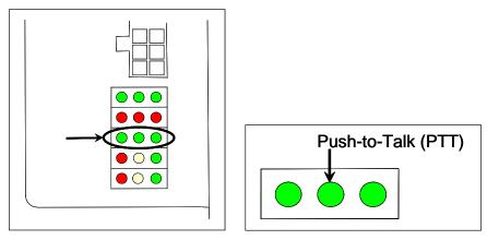
If this LED isn't lit, the system's ability to send a message or tone to the radio might be inhibited. This can happen when one uses the **Radio Inhibit option** on the System Functions menu. If the radio is inhibited, the results of this check are invalid.
