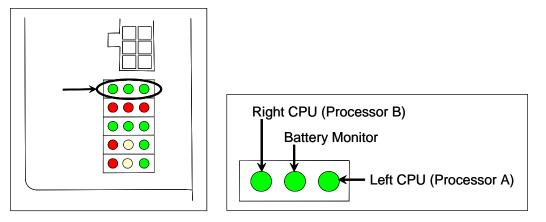
The top row of green LEDs indicates the condition of the CPUs and the battery on the Processor board. If both CPUs are running their programs correctly, their LEDs pulsate (that is, repeat the cycle off, dim, bright, dim). If a program isn't operating as expected, the LED for the affected CPU blinks on and off, is lit solid, or isn't lit at all.
