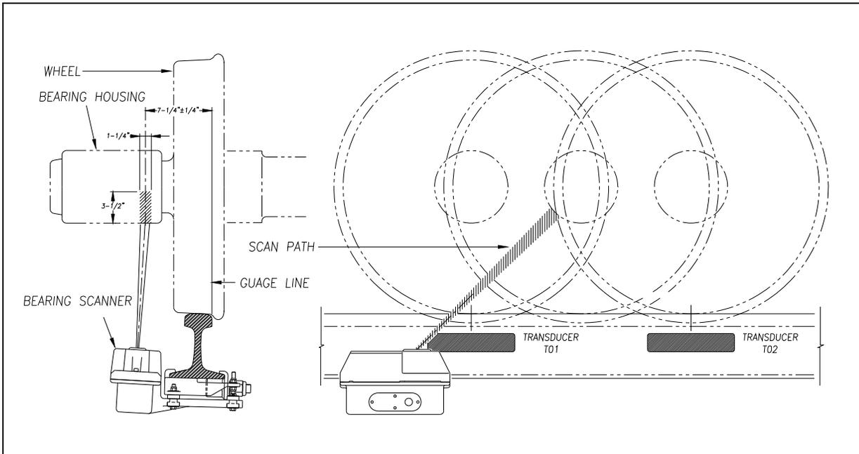
The **type3** bearing scanners are aligned to scan the bottom 3.5 inches (8.9 centimeters) of the bearing housing, about 7.25 inches (18.4 centimeters) from the gauge line.
