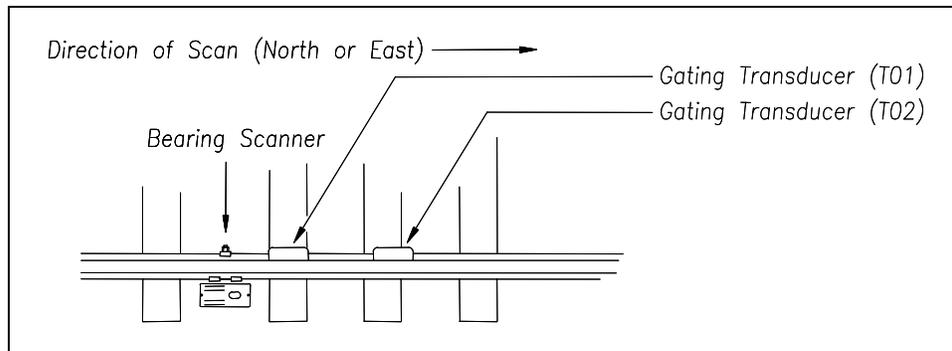
The signals from these gating transducers indicate to the system that passing wheels are in view of the scanners. Furthermore, the speed of the train is determined by using the known distance between TO1 and TO2 versus the time required for a given wheel to pass over them.
