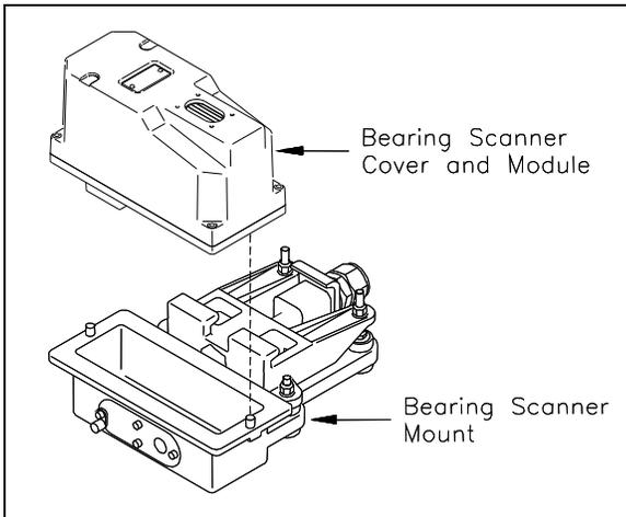
To replace a **type2/type3** bearing scanner cover-and-module assembly:
