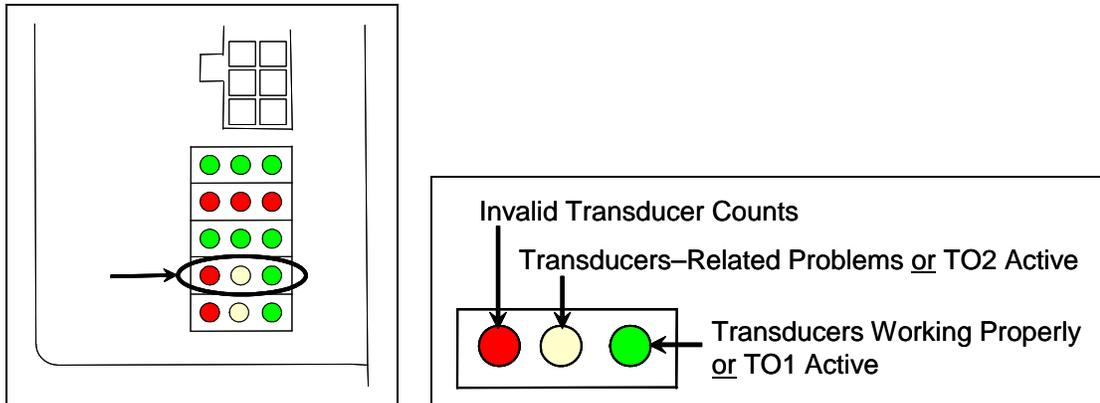
On the Interface board (in the Controller module), the transducer signals undergo RF filtering and amplification with a gain of 30. For validation, the amplified signals are fed into comparators, which create 5-VDC pulses lasting the period of time that the amplified signals remains above 620 millivolts. Processor-A (on the Processor board) receives these 5-VDC pulses through ports PA0 (TO1) and PA1 (TO2).
