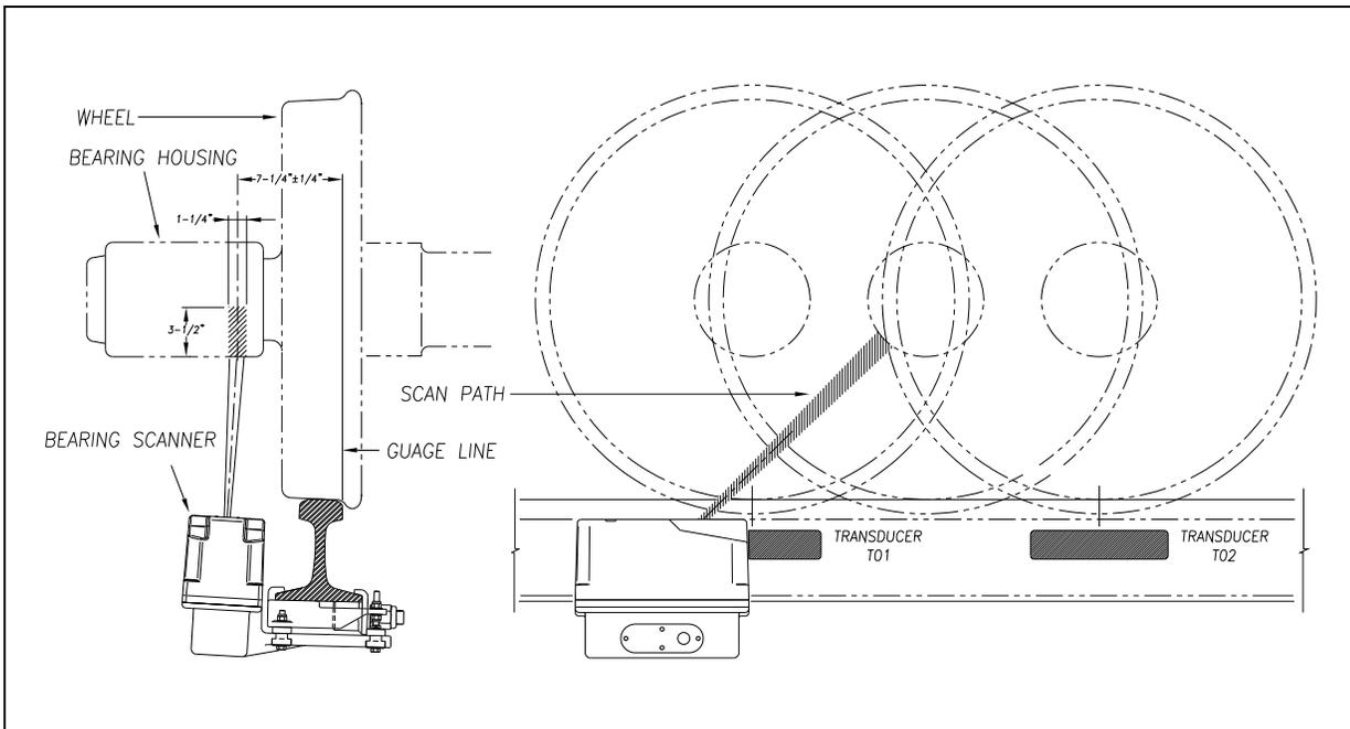
Bearing temperatures are sampled for a short period before the gate opens, to support detection of Pyrometer Saturation alarms, and while the gate is open.
