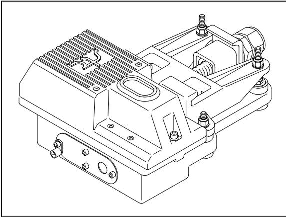
An assembled **type3** bearing scanner looks like this.
