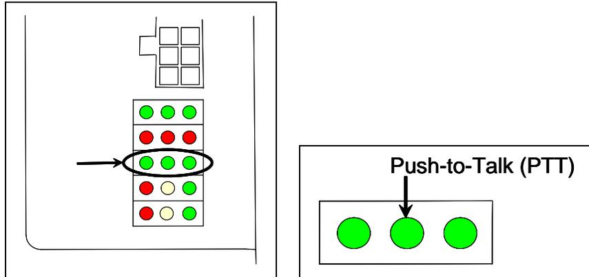
If this LED isn't lit, the system's ability to send a message or tone to the radio might be inhibited. This can happen when one uses the **Radio Inhibit option** on the System Functions menu. If the radio is inhibited, the results of this check are invalid.
