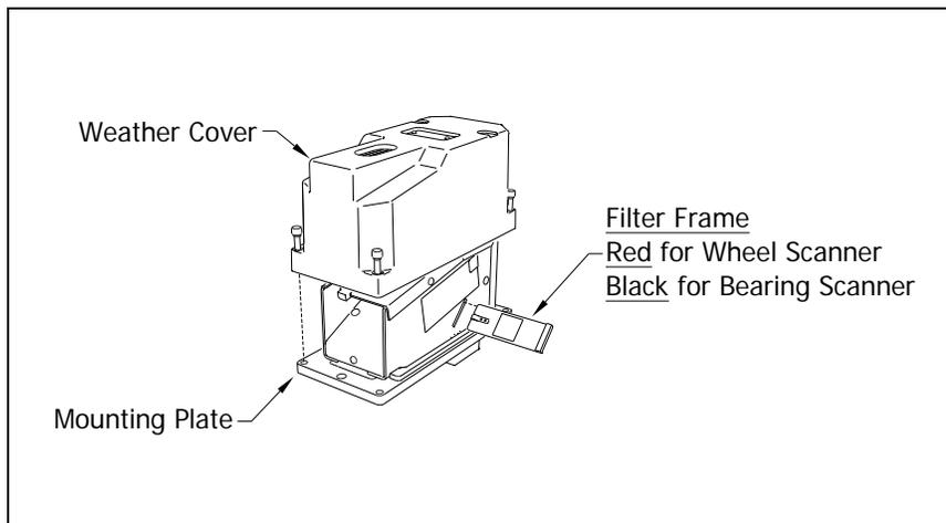
You'll need to remove the weather cover before you can replace the filter frame. Four socket-head-cap screws attach the weather cover to the mounting plate. Before continuing, be sure that the **black** filter frame is securely in place and that the four socket-head-cap screws on the weather cover are completely tight.
