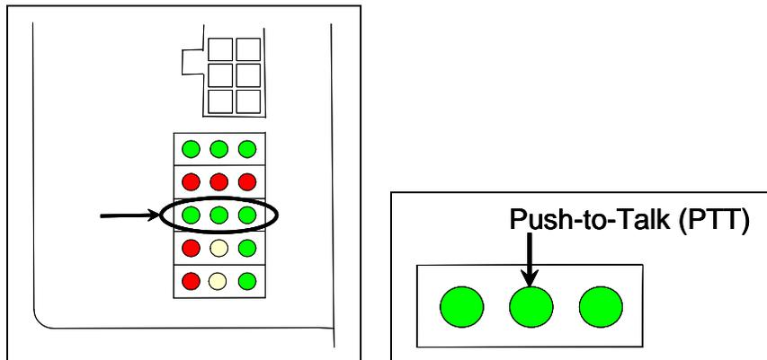
If this LED isn't lit, the system's ability to send a message to the radio might be inhibited by the **Radio Inhibit option** on the System Functions menu. If the radio is inhibited, the results of this check are invalid.
