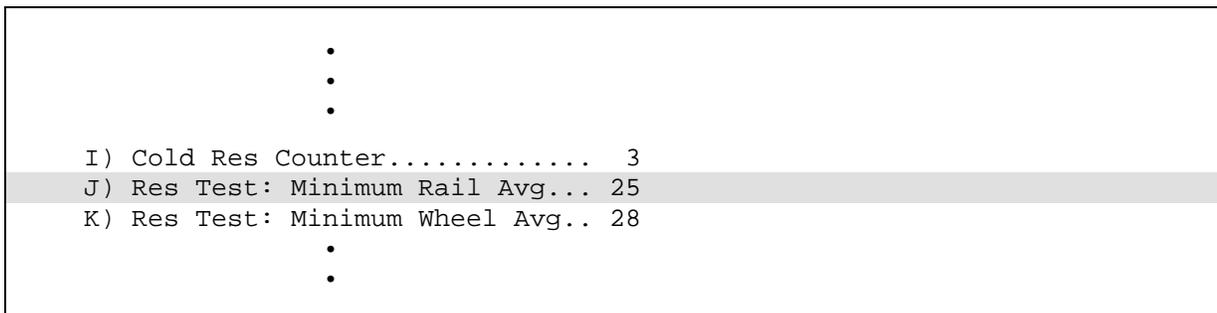
If the average heats are less than the value set by the **Resistor Test Minimum Rail Average option**, the system generates a Cold Resistor alarm.
