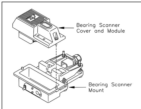
The figure below shows the major parts of a **type3** bearing scanner.
