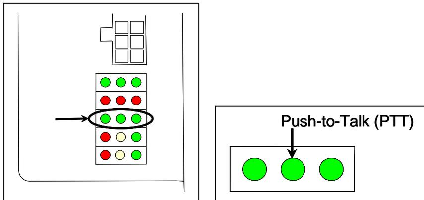
If this LED isn't lit, the system's ability to send a tone to the radio might be inhibited by the **Radio Inhibit option** on the System Functions menu. If the radio is inhibited, the results of this check are invalid.
