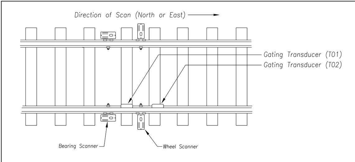
The **type2** wheel scanners are aligned to scan about 4 inches (10.2 centimeters) above the rail.
