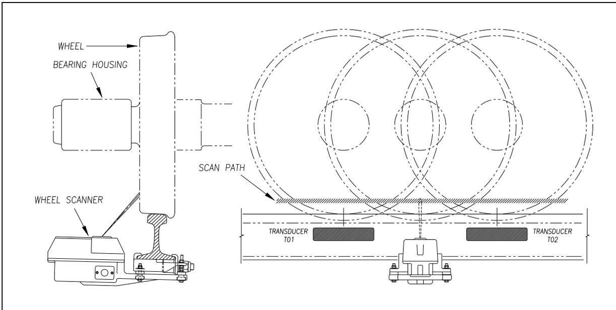
The **type3** wheel scanners are aligned to scan about 4 inches (10.2 centimeters) above the rail.
