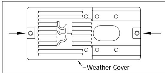
The **type3** wheel scanner has six. Four that attach the weather cover to the mounting plate and two that attach the mounting plate to the mount.
