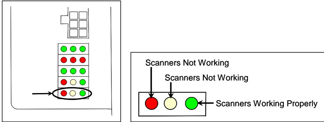
The bottom row of LEDs indicates the operational condition of the bearing and wheel scanners when the system is at rest (that is, when a train isn't present at the site). Several conditions are monitored and logged.
