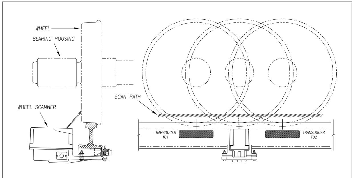
The SmartScanNG system checks for hotwheels during the scanning process.
