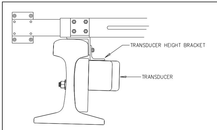
The fixture should be snug against the top and gauge of both rails. This may be impossible if the transducer body is less than 1-9/16 inches (3.97 centimeters) below the top of the rail or if the transducer body isn't parallel to the top of the rail.
