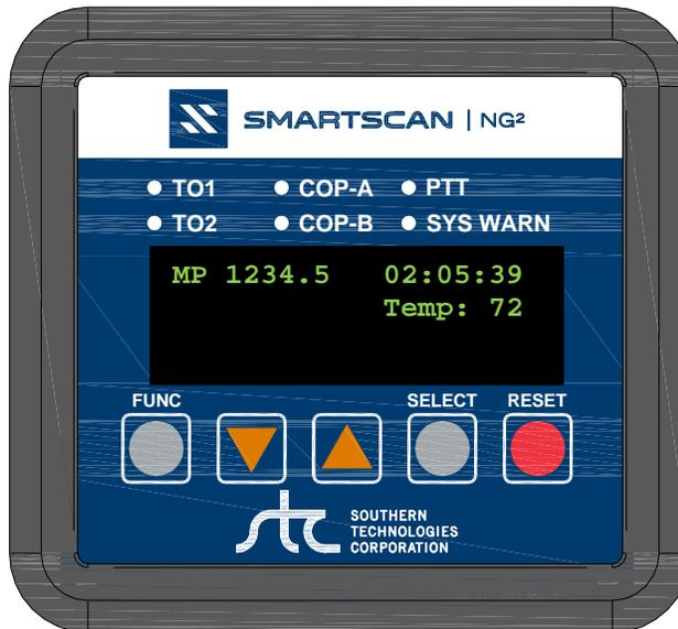
The COP-A and COP-B LEDs indicate the general health of each processor. If both the analyzer processor and the communications processor are running their programs correctly, their LEDs blink on and off. If a program isn't operating as expected, the LED for the affected processor is lit solid or isn't lit at all.
