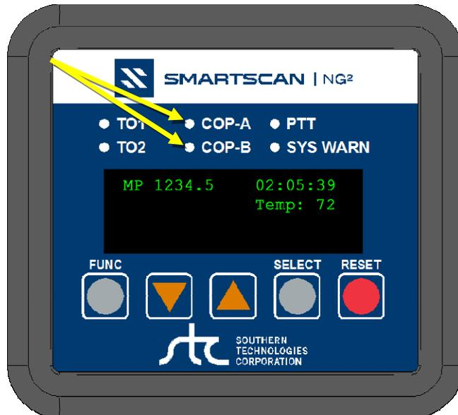
The COP LEDs indicate the condition of the CPUs. If both CPUs are running their programs correctly, their LEDs blink on and off. If a program isn't operating as expected, the LED for the affected CPU is lit solid or isn't lit at all.
