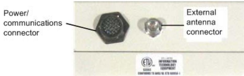
**Figure 4-2 Back of Encompass 4 Reader Showing Antenna Connector**
