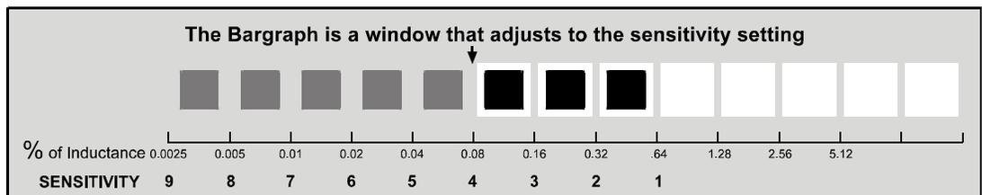
The bargraph, below, has the same vehicle in the loop zone causing the same inductance change as above. Since the sensitivity setting was increased to Level 7, six segments are now displayed. If the bargraph displays 5 or 6 segments for a vehicle in the loop and motorcycles are not a concern, the sensitivity has been set to the proper range.
