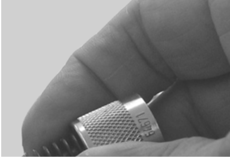
Figure 3–2 Connect RF N-type Load or Attenuator to Reader Cable End
