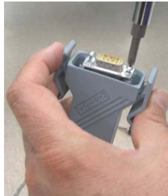
Figure 11-5 Securing Terminal Strip into Connector Housing
