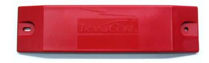
The PT5780 Permissions Tag is used to configure the AP4118 Rail Tag Programmer. Multiple programmer parameters, such as programmer control number, serial number, and tag programming certification expiration date are transferred from the PT5780 to the AP4118 via the RF link. The AP4118 validates the PT5780 data and, if valid, stores the data in the programmer's non-volatile memory.
