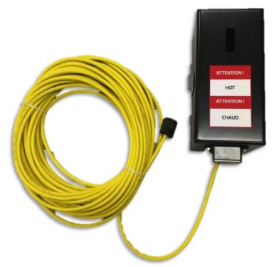
The 2500-575 Heated Auxiliary Scanner Cover is designed to prevent accumulations of snow and ice on top of a Type III bearing or wheel scanner during extended periods of low ambient temperatures in inclement weather. **The covers are intended to be used seasonally!** As such they should be removed and stored in the signal bungalow when sustained ambient temperatures are above 40 degrees F.
