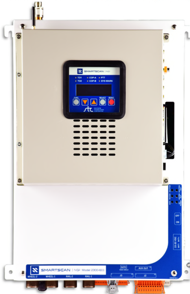
Figure 2 - SmartScanNG 2 Controller Module and SmartScanNG 2 Chassis
